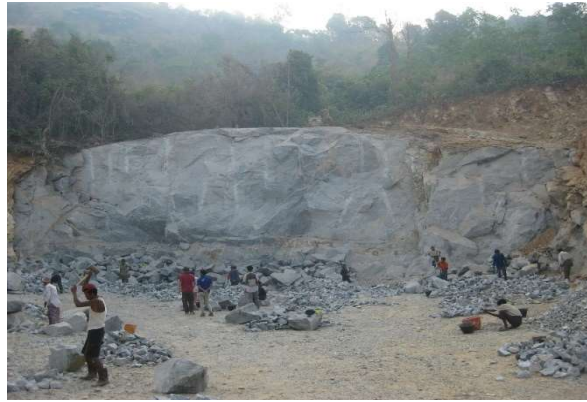
Figure 28. Biotite granite is excavated for construction and decorative stones at Daminzeik Quarry.
